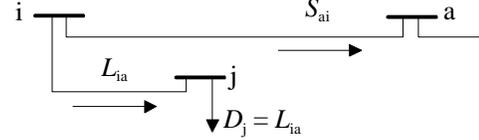
Fig. 4. Decoupled power flow of the line i-a.
