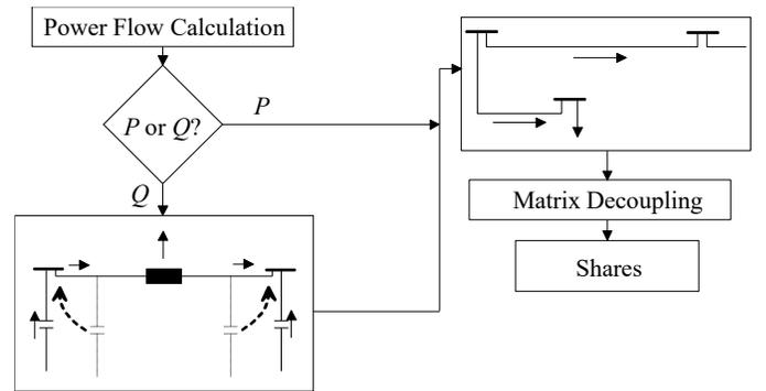
Fig. 8. Algorithm of the proposed method of power-flow tracing.
