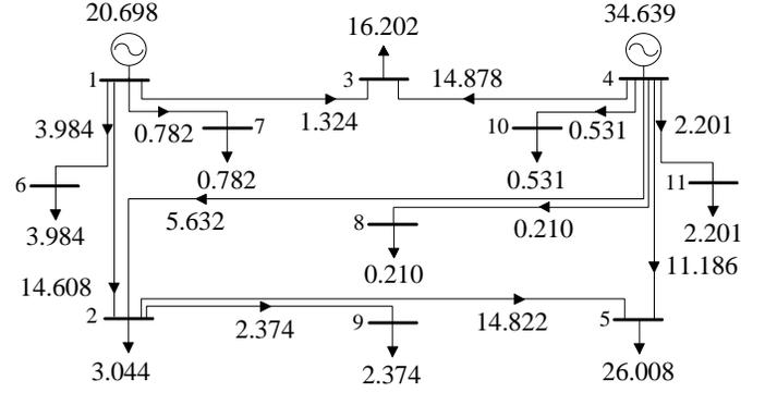
Fig. 17. 5-bus test system with the reactive-power flows in MVar modified by the improved TGDF method.
