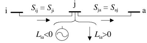
Fig. 2. Additional node on the line  $i$ - $a$ .
