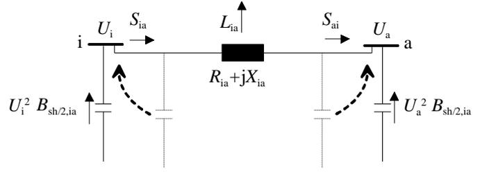
Fig. 3. Equivalent model of the line i-a.
