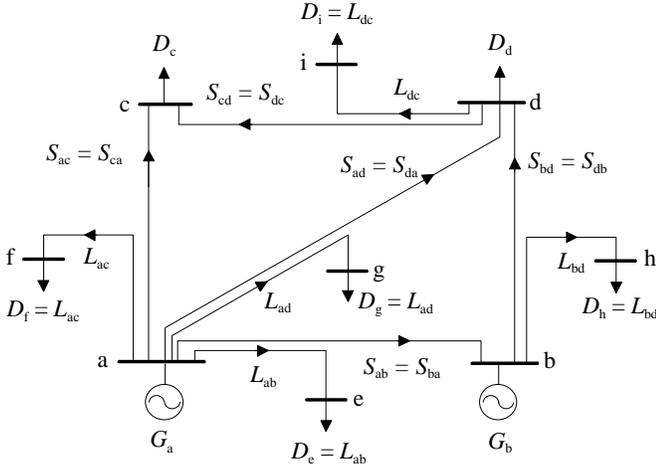
Fig. 6. Decoupled 4-bus test system.
