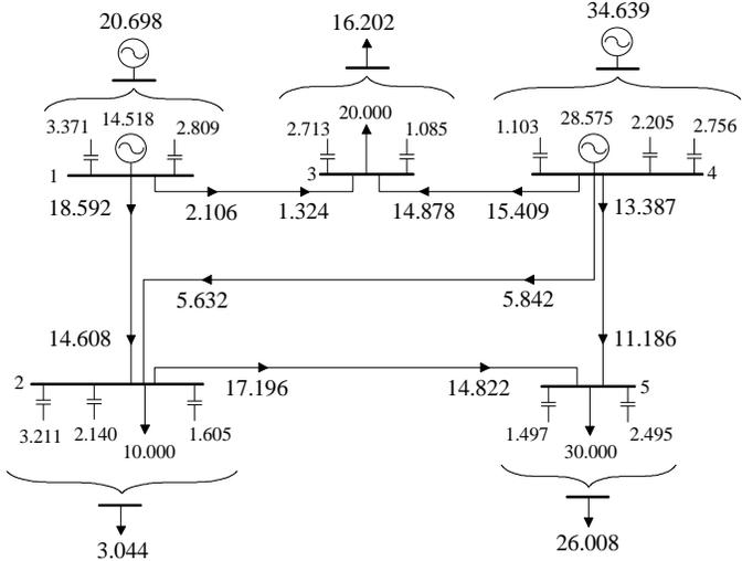
Fig. 16. Reactive power flows in MVar after introducing the equivalent model of a line.
