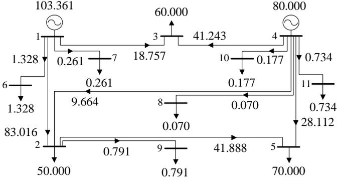
Fig. 15. 5-bus test system with the active-power flows in MW modified by the improved TGDF method.
