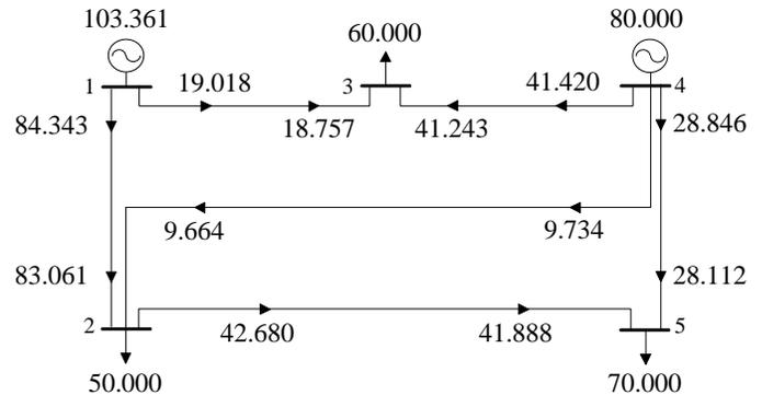
Fig. 12. 5-bus test system with the active-power flows in MW.
