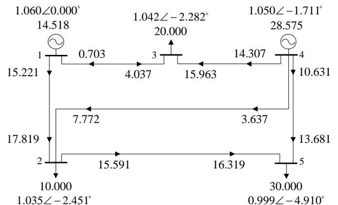
Fig. 13. 5-bus test system with the nodal voltages and the reactive-power flows in MVAR.
