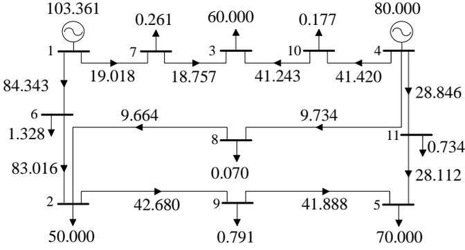
Fig. 14. 5-bus test system with the active-power flows in MW modified by the TGDF method.
