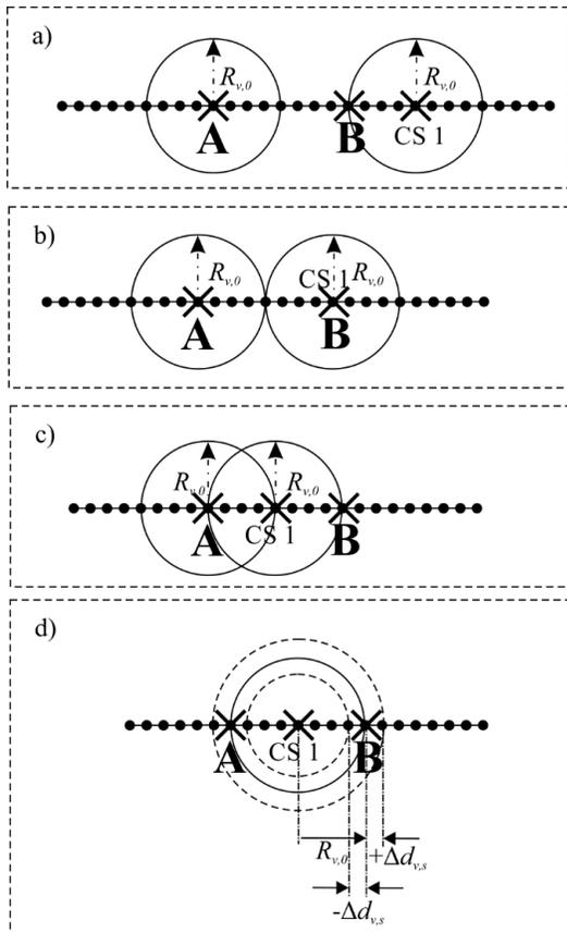
Figure 1: Charging reliability principle and uncertainty distance with regards to the EDV driving range
