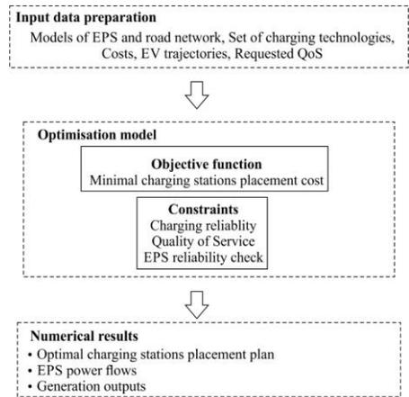
Figure 1 Flow-chart presenting the optimal CSs placement planning procedure with the EPS reliability check
