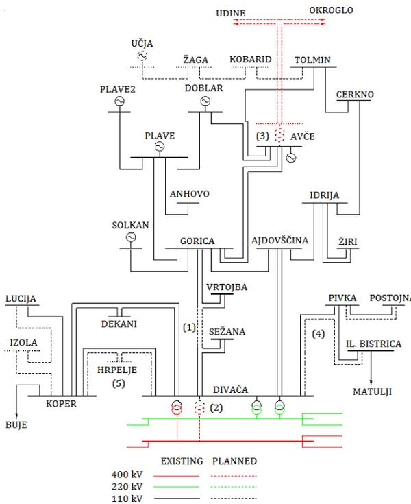
Fig. 25. Model of grid and required development candidates by 2020 [17]
