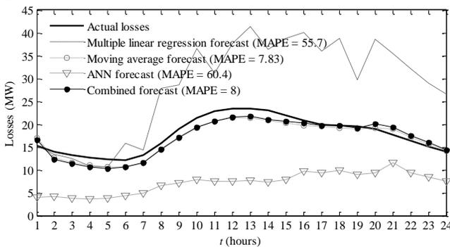
Fig. 15. Transmission losses for the Slovenian power system for the chosen day for the Slovenian power system where larger amounts of weather data are missing.
