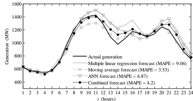
Fig. 11. Comparison of generation forecasting results for the chosen day for the Slovenian power system.
