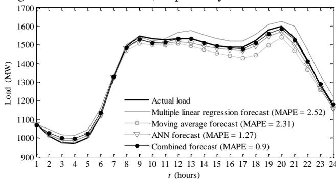
Fig. 8. Comparison of load forecasting results for the chosen day for the Slovenian power system.
