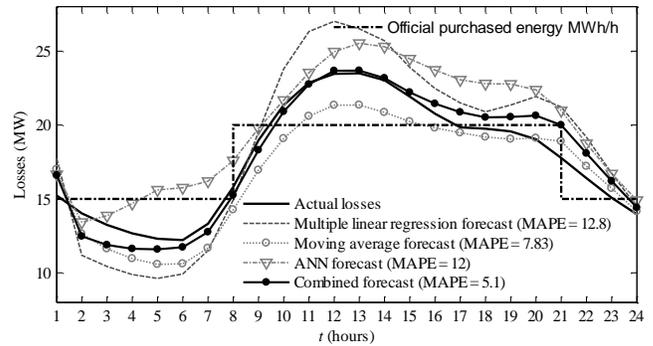
Fig. 12. Transmission losses for the Slovenian power system for the chosen day for the Slovenian power system.
