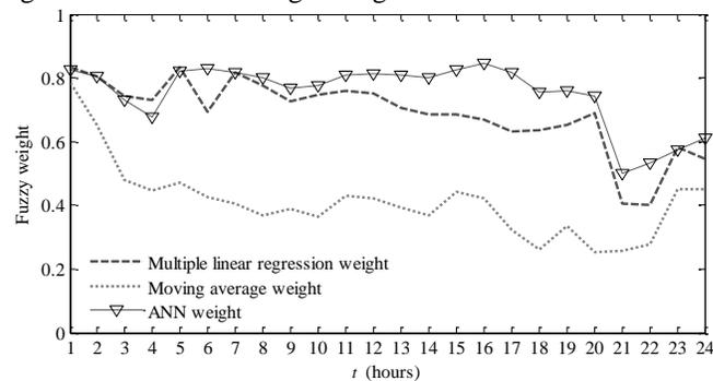
Fig. 10. Fuzzy weights for individual forecasting methods for the chosen day.
