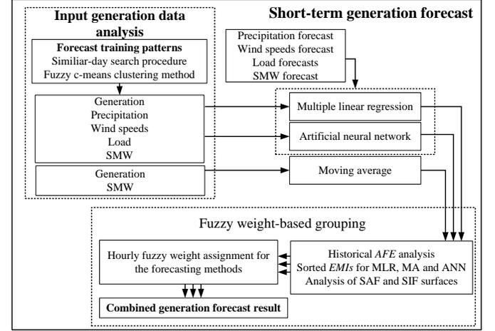
Fig. 7. Flow chart for the short-term generation forecasting.
