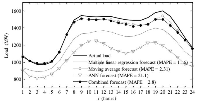
Fig. 13. Comparison of load-forecasting results for the chosen day for the Slovenian power system with missing or incomplete weather data.
