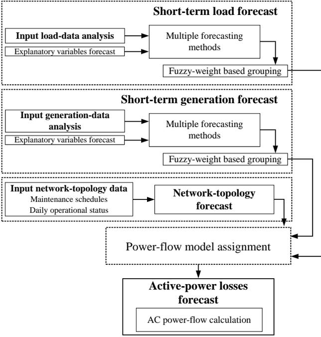
Fig. 1. Flow chart for the transmission-losses forecast method.
