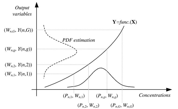
Fig. 4. Principle of PE methods.
